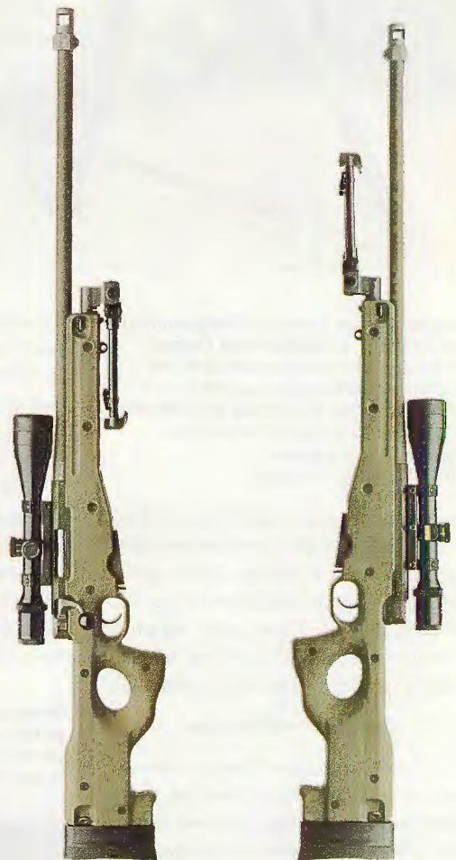
Right side view of AW sniper rifle. Bolt lift upon opening is only 60 degrees. Total bolt throw is 4.2 inches, which allows the operator to maintain his cheek-weld on the stock while manipulating the bolt and thus observe the target during reloading.
